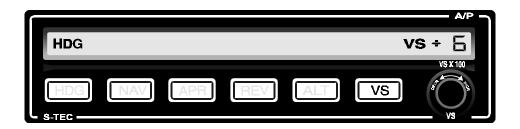
The + (positive) symbol annunciation indicates a *climb* vertical speed selection. Clockwise rotation of the **VS** knob increases the rate of climb and counter clockwise rotation decreases the rate of climb to 0. The - (negative) symbol annunciation indicates a *descent* vertical speed selection. Counter clockwise rotation of the **VS** knob increases the rate of descent and clockwise rotation decreases the rate of descent to 0. Maximum selectable VS limits are  $\pm$  1600 FPM.
