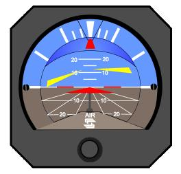
For proper flight technique, the system presentation requires the pilot to roll and pitch the aircraft toward the steering command bars until the delta-shaped reference is tucked into the steering command bars, indicating that commands have been satisfied. For example, if the display is up and left, the pilot would be required to establish a left turn, pitch-up attitude.
