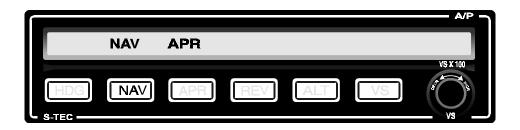
If the course needle is at full-scale deviation, the autopilot will establish a 45° intercept angle. As the aircraft approaches the localizer course, the autopilot senses the closure rate, and gradually, smoothly shallows the intercept angle. The point at which this turn begins is variable, depending on the aircraft position and closure rate to the course. However, the turn will always begin between 100% (full-scale) needle deflection and 20% of full-scale.
