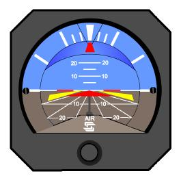
This system, which integrates both the roll axis and pitch axis, offers synchronized display of the flight profile. It is automatically activated when the autopilot is engaged. A Flight Director provides a visual indication of how accurately the pilot or autopilot is tracking the commands of the active mode of operation.
