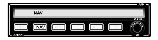
Engage the **NAV** mode. If the course needle is at full-scale deviation, the autopilot will establish a 45° intercept angle. As the aircraft approaches the selected course, the autopilot senses the closure rate, and gradually, smoothly shallows the intercept angle. The point at which this turn begins is variable, depending on the aircraft position and closure rate to the course. However, the turn will always begin between 100% (full-scale) needle deflection and 20% of full-scale.
