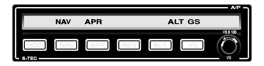
Glideslope capture is indicated by extinguishing of the *ALT* annunciation.
