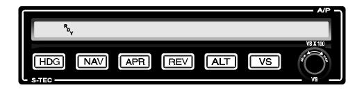
Should a fault be detected, the *FAIL* annunciation will remain on at the conclusion of the test and the autopilot can not be engaged.
