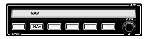
If the course needle is at full-scale deviation, the autopilot will establish a 45° intercept angle. As the aircraft approaches the selected course, the autopilot senses the closure rate, and gradually, smoothly shallows the intercept angle. The point at which this turn begins is variable, depending on the aircraft position and closure rate to the course. However, the turn will always begin between 100% (full-scale) needle deflection and 20% of full-scale.
