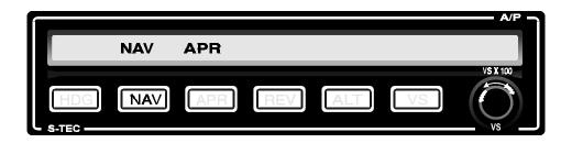
If the course needle is at full-scale deviation, the autopilot will establish a  $45^{\circ}$  intercept angle. As the aircraft approaches the localizer course, the autopilot senses the closure rate, and gradually, smoothly shallows the intercept angle. The point at which this turn begins is variable, depending on the aircraft position and closure rate to the course. However, the turn will always begin between 100% (full-scale) needle deflection and 20% of full-scale.
