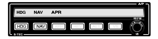
The selected heading will now be flown until the autopilot computes that an on course turn must be made to minimize overshoot at the point of intercept. At the time the on course turn begins, the **HDG** mode will extinguish and you must move the heading bug to match the localizer course. This will allow the autopilot the full range of cross wind correction during **NAV**, **APR** track mode.
