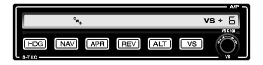
Depress and hold the **Control Wheel Steering** switch located on the aircraft's control wheel. The *CWS* and *VS* modes will annunciate and *RDY* will extinguish. Position the aircraft in the desired roll and pitch attitude. Note: Aircraft vertical speed x 100 will be displayed in the Programmer/Computer Annunciator window directly above the VS selector knob. Example: +6 equals 600 FPM rate of climb.
