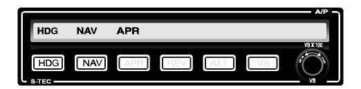
The selected heading will now be flown until the autopilot computes that an on course turn must be made to minimize overshoot at the point of intercept. At the time the on course turn begins, the **HDG** mode will extinguish.
