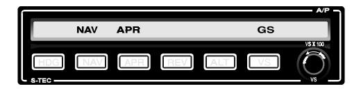
NOTE: IF VECTORED TO INTERCEPT THE LOCALIZER TOO CLOSE TO THE GLIDESLOPE INTERCEPT POINT, RESULTING IN LESS THAN 60% GS NEEDLE DEVIATION WHEN ON COURSE, THE SYSTEM WILL NOT AUTOMATICALLY ARM THE GLIDE-SLOPE. MANUAL ARMING MUST THEN BE FOLLOWED.
