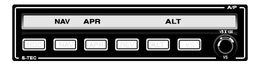
Glideslope arming will occur when the above conditions have existed for 10 seconds. Illumination of the GS annunciator will occur, indicating arming has been accomplished. The ALT annunciator remains on.
