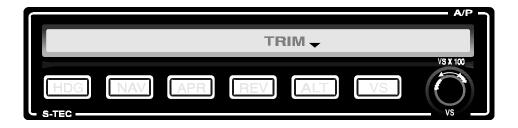
If the trim master switch is OFF or a failure has occurred in the autotrim, the system will automatically revert to "Pitch Trim Indicator" mode of operation.
