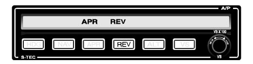
If the course needle is at full-scale deviation, the autopilot will establish a 45° intercept angle. As the aircraft approaches the localizer course, the autopilot senses the closure rate, and gradually, smoothly shallows the intercept angle. The point at which this turn begins is variable, depending on the aircraft position and closure rate to the course. However, the turn will always begin between 100% (full-scale) needle deflection and 20% of full-scale.
