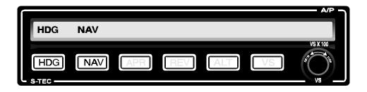
The selected heading will now be flown until the autopilot computes that an on course turn must be made to minimize overshoot at the point of intercept. At the time the on course turn begins, the *HDG* mode will extinguish and you must move the heading bug to match the selected radio course. This will allow the autopilot the full range of cross wind correction during *NAV* track mode.
