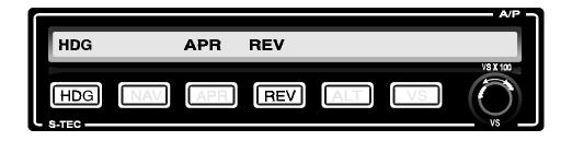
The selected heading will now be flown until the autopilot computes that an on course turn must be made to minimize overshoot at the point of intercept. At the time the on course turn begins, the *HDG* mode will extinguish and the heading bug must be moved to match the localizer back course inbound. This will allow the autopilot the full range of cross wind correction during *NAV*, *APR* track mode.
