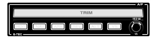
The S-TEC trim system is designed to accept any type of single failure - mechanical or electrical - without uncontrolled operation resulting. To ensure that no hidden failures have occurred, conduct a trim preflight check prior to every flight.
